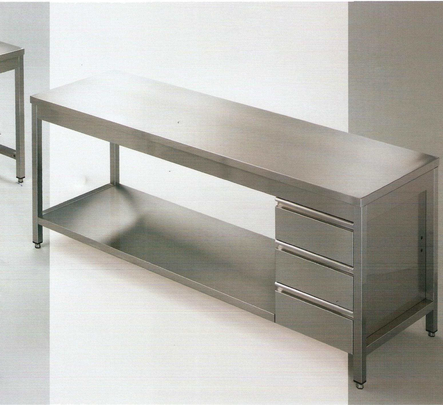
Working benches are made entirely of INOX 18/10 AISI 304 with ergonomic design and are offered in different lengths from 70cm till 220cm with formation every 10cm. They are being disposed with or without lower or intermediate self and there is the possibility of placement vertical drawers and bottom hung container.
